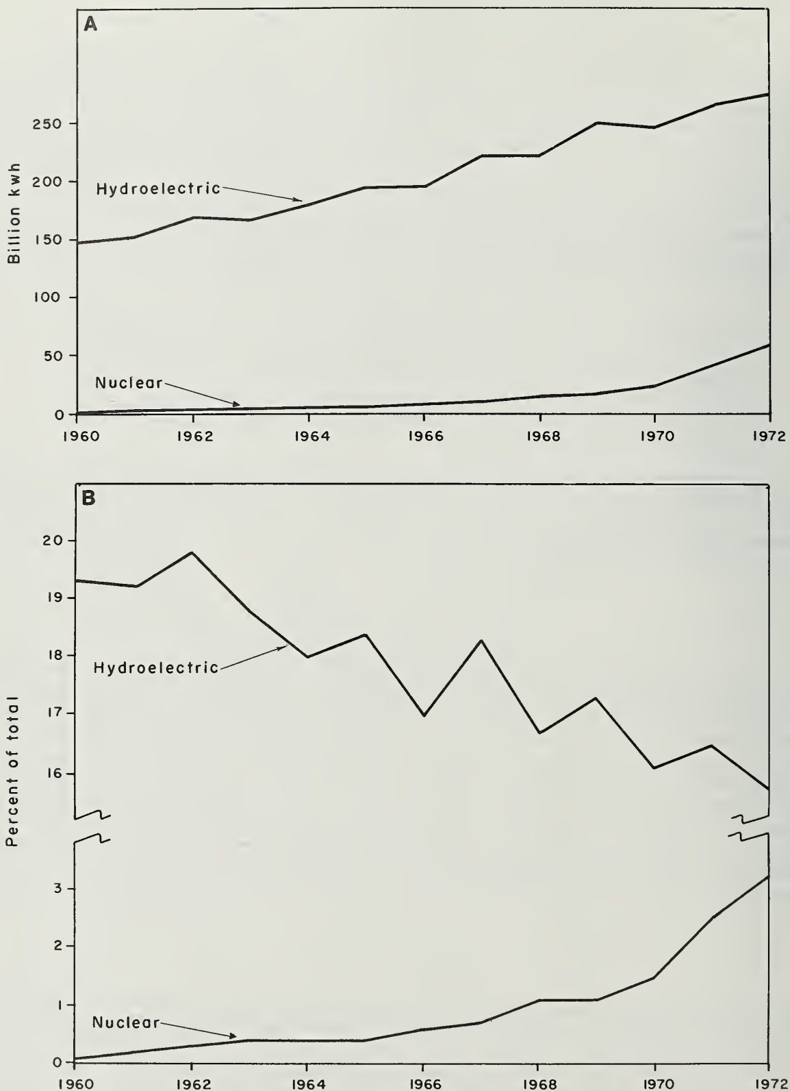
Fig. 9 - A. Electric power output by utilities from hydroelectric and nuclear plants. B. Percentage of total electric power output of utilities that is provided by hydroelectric and nuclear plants.
